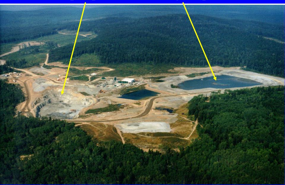
Quinsam backfills potentially ARD generating coarse coal rejects into a flooded pit
