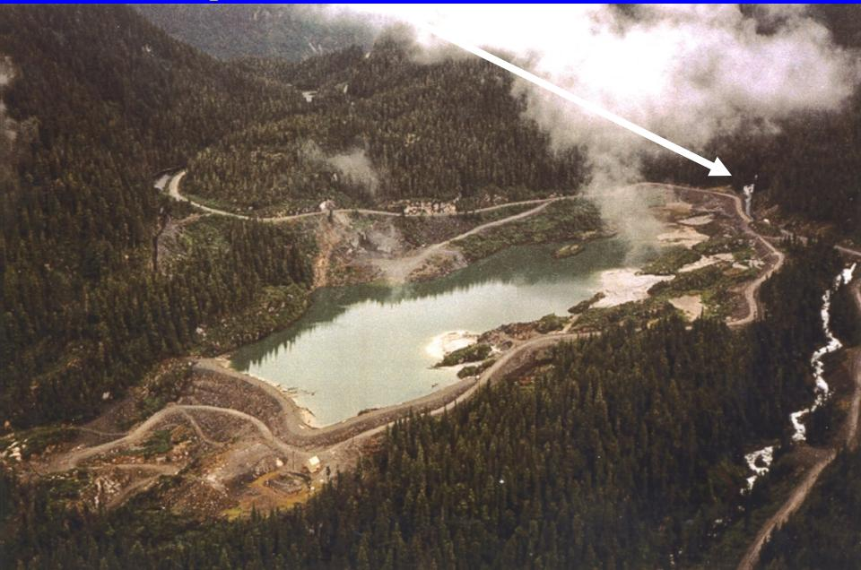
**Re-diverting stream** flow through the impoundment and over tailings would avoid the risks and maintenance associated with the Cascade Creek diversion.
