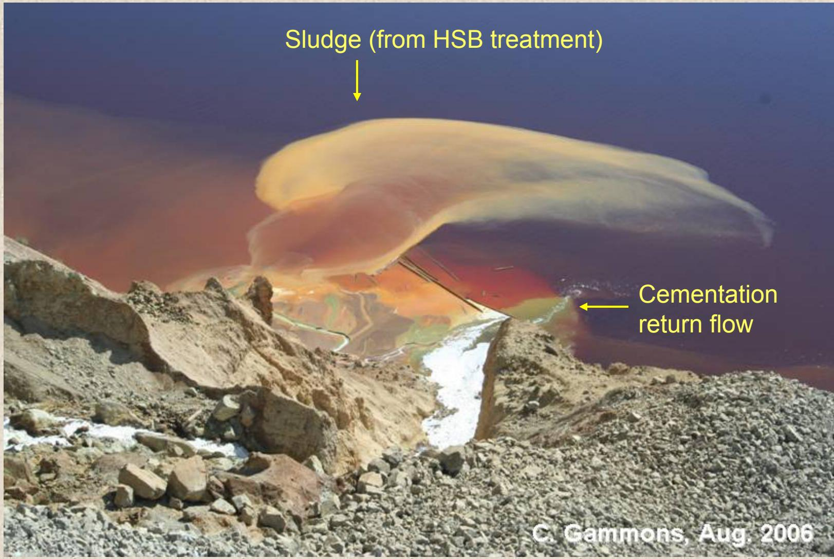
Copper cementation circuit and lime treatment
