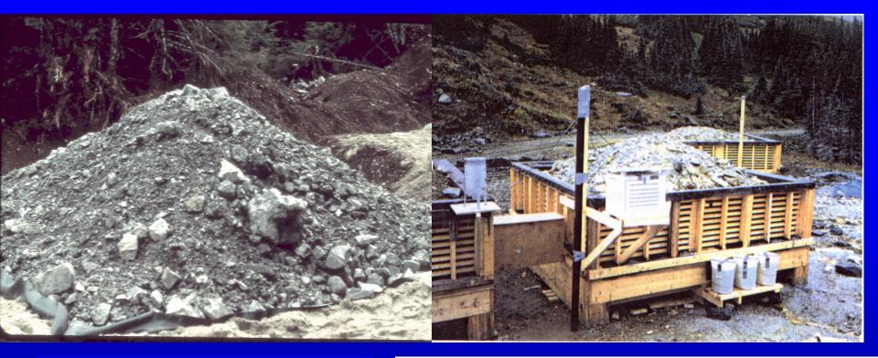
Field test cells or pads measure influence of site conditions on weathering and drainage chemistry.
