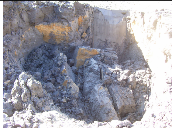
Collapsed test pit, June 10. Note the cohesion within the mass, with no indications of liquefaction-type behaviour.
