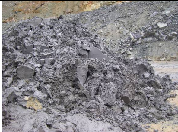
Pile of excavated material after 3.5 hours. Note the cohesion within the material, with no indications of liquefaction-type behaviour under high strains imposed by the excavation process.
