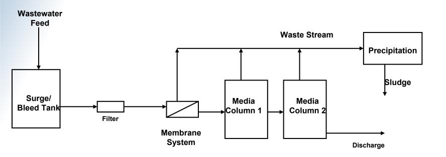
Block diagram of Asarco's membrane separation process
