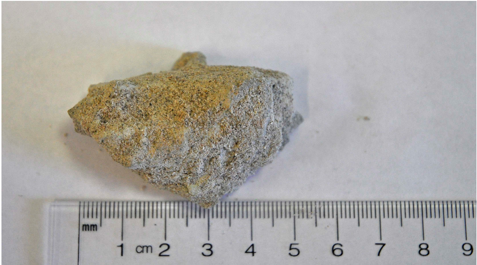
Photograph of Scorodite Scale from Leaching Process Reactor Tank
