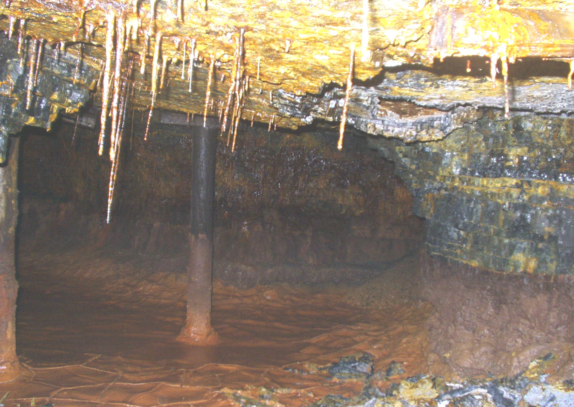
Glace Bay - MacKay's Corner "bootleg" workings and AMD formation 2004
