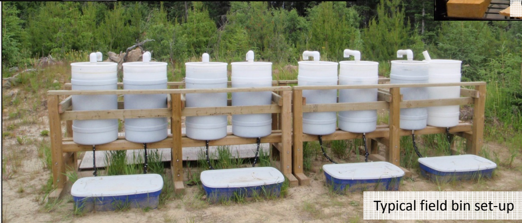
Humidity cells; from ASTM D5744
