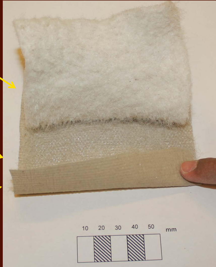
GTX of GCL - Bentonite removed
