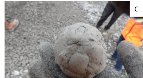
Forming of a ball to test the paste rock cohesion
