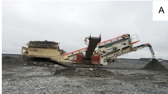
Belt sieving the rough mix and spilling at a height of 2 m
