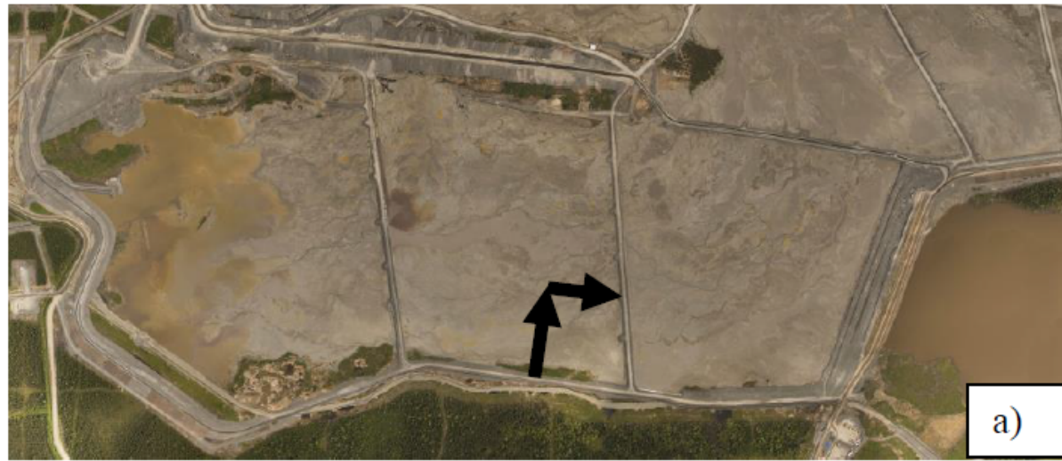
Figure 3 – a) Photo of the southern part of the Canadian Malartic tailings impoundment with the approximate location of the two new waste rock inclusions (arrows) that will be built for this project; b) Schematic view of the waste rock inclusions in the impoundment
