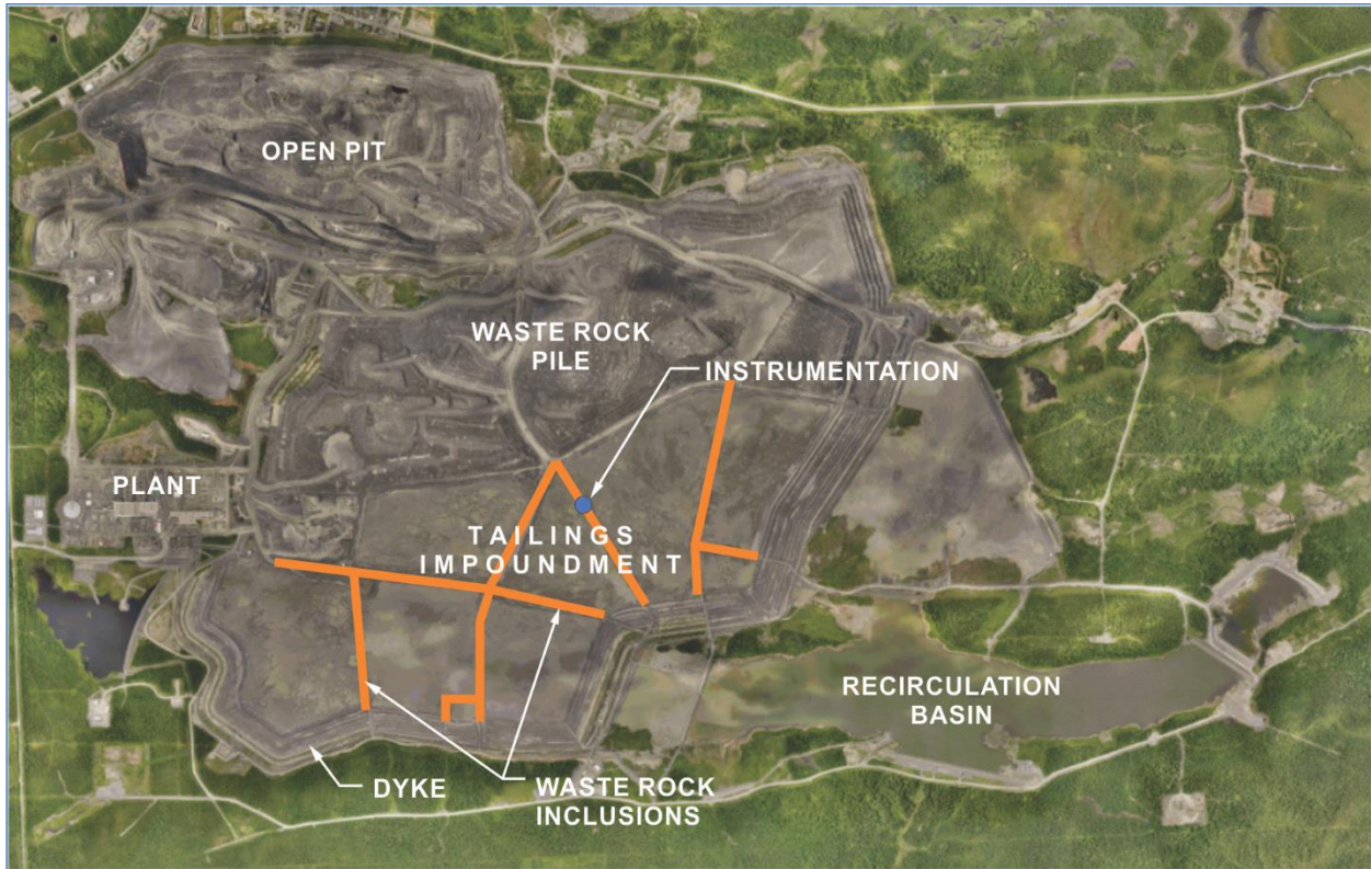
Figure 4. Aerial photograph of the Canadian Malartic Mine with waste rock inclusions shown in orange (from 2015 aerial photograph of site by Canadian Malartic Mine).
