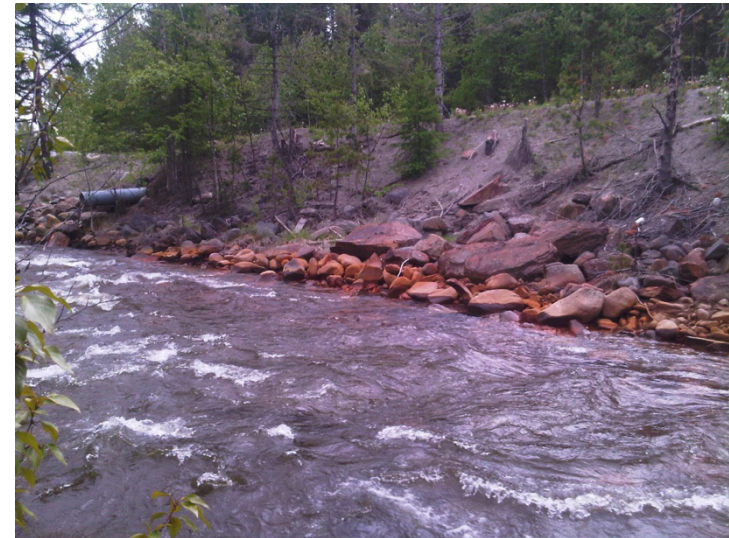
Precipitate staining from ARD bypass identified in 2012
