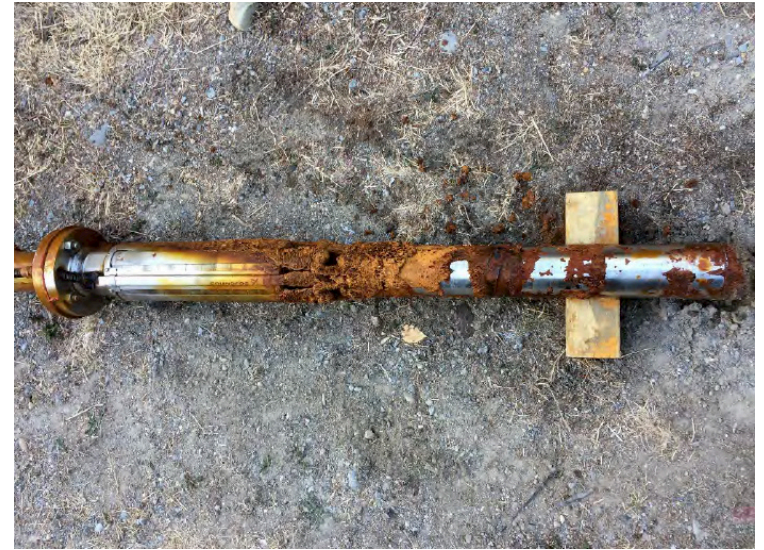
Precipitate build up on deep aquifer pump
