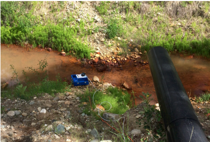
Dye Testing in Siliceous Pond Collection Ditch
