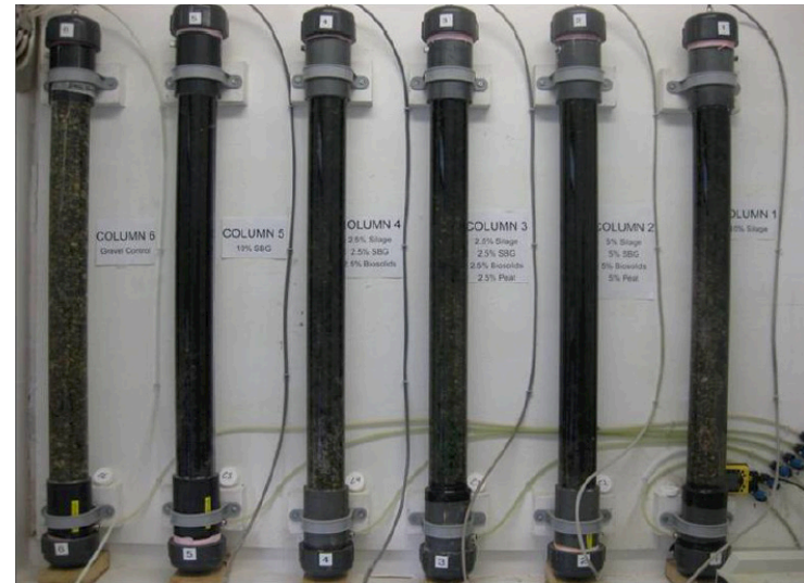
Bench-scale column set-up, upflow configuration
