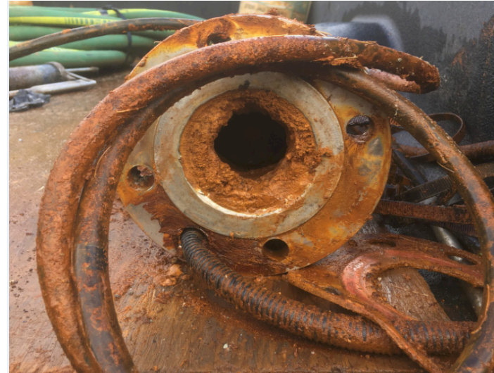
Build up in Lower Mine Yard pump discharge piping
