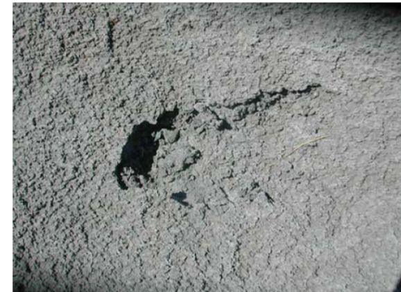
Figure 3.104 Salt crust development at Mt Keith, TSF 1 (November 2002)
