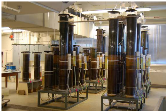
Photo 1: Overview of Column Set-Up.
