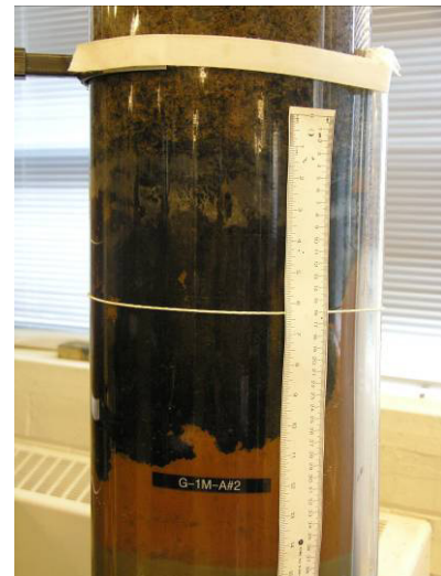
Photo 2: Close-up of black precipitate at tailings/organic interface.
