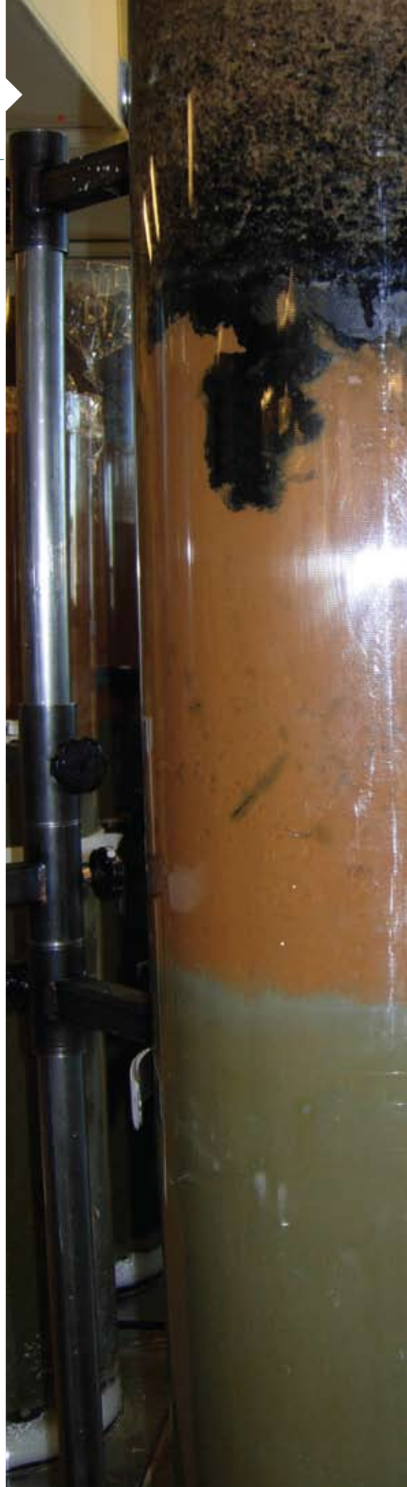
CLOSE-UP OF EVIDENCE OF SULPHATE REDUCTION IN LEACHING COLUMNS AT CANMET-MMSL. INSET: OVERVIEW OF LEACHING COLUMNS AT CANMET-MMSL.
