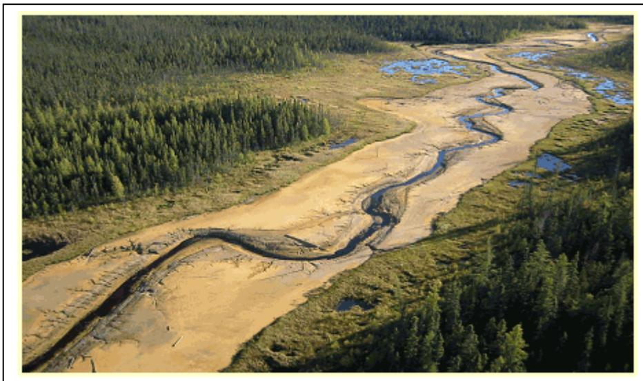
The waste deposited in the tailings impoundment without adequate containment spread out around the deposition zone and along Ruisseau Manitou over a distance of
