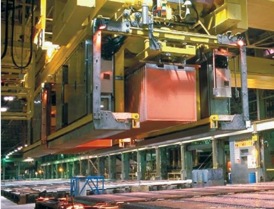
Copper sheets sometimes detached from the blank prematurely and fell to the machine floor.
