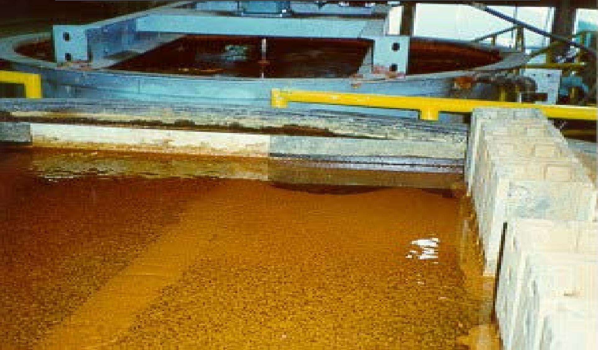
Both Sulphurets (pictured here) and Eskay Creek added lime to acidic waste rock to neutralize the pH of waste rock prior to flooding. In both cases, the waste rock was exposed during exploration.
