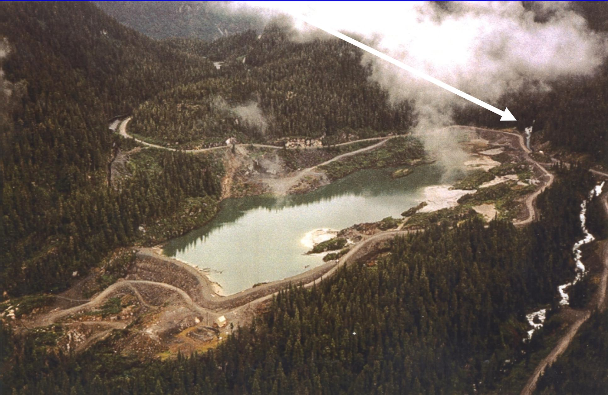
Re-diverting stream flow through the impoundment and over tailings would avoid the risks and maintenance associated with the Cascade Creek diversion.
