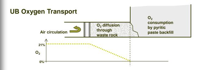
Assumption: Rate limiting step is diffusion through waste rock
