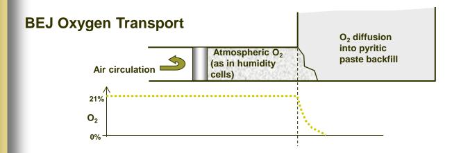
Assumption: Rate limiting step is diffusion into backfill
