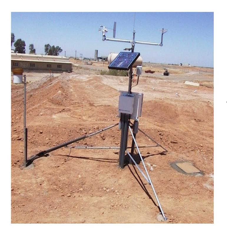
Installed weather station & datalogger with cellular telecommunications.
