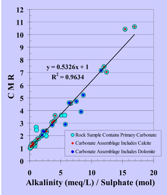
• Excess Alkalinity produced from water dissolution is directly related to the elevated CMR
