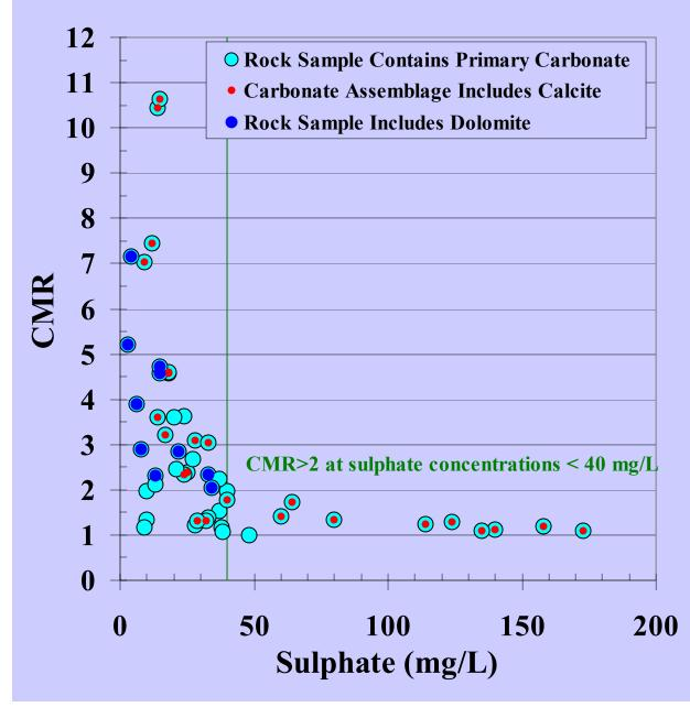
•Sulphide Oxidation produces > 40 mg/L SO<sub>4</sub> CMR values remain < 2.0
