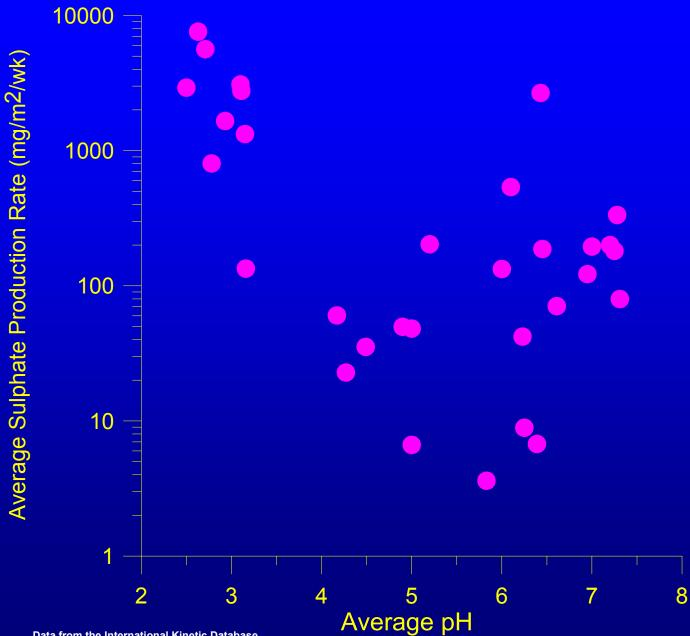
For example, the **International Kinetic Database contains Minewall-station** data from several minesites. The compiled data (left) shows a large range in unit-area rates of sulphate production.
