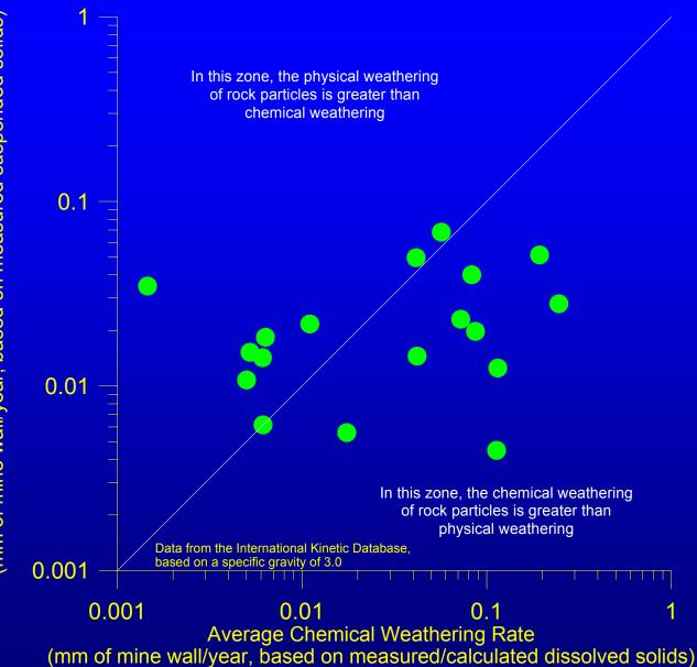
When the weathering rates are converted to mm of mine wall/year, average rates of both physical and chemical weathering are typically between 0.005 to 0.1 mm/year. This is not a major rate, but over 100 years of operation and closure becomes 0.5-10 mm.
