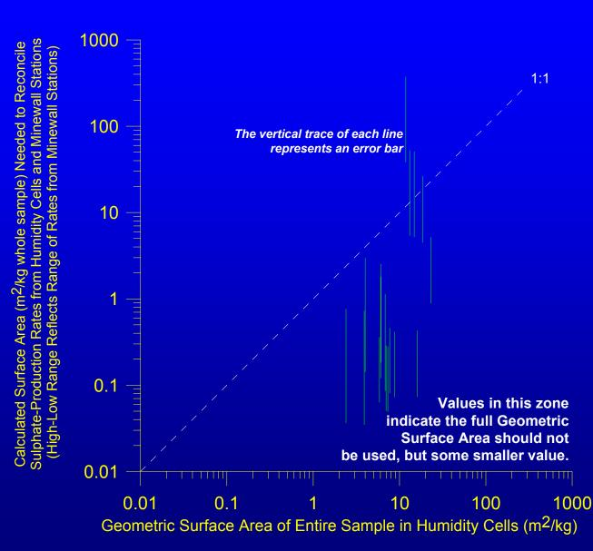
For most comparisons of actual cells rates to actual Minewall rates, the Geometric Surface Area (GSA) was too high for accurate conversions. Instead, a smaller surface area was justified.
