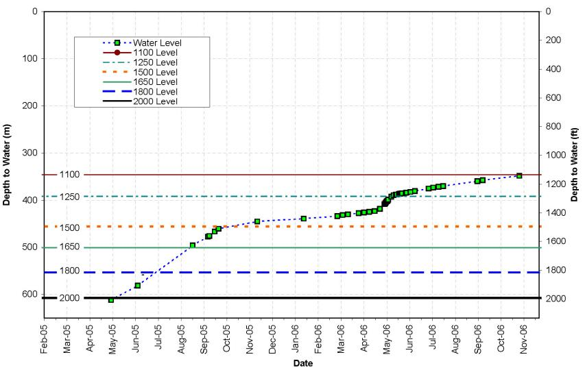
C-Shaft Water Level vs. Time
