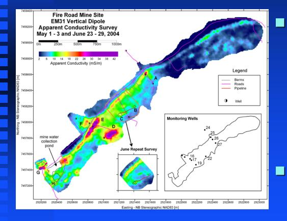
Conductivity highs at B and C coincide with the discharge location of the sludge pipeline in 2002 and 2003. Note seasonal variation.
