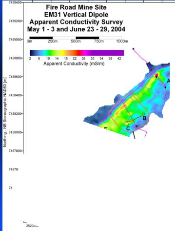
$\blacksquare$  Note the scale. Electrical conductivities in waste rock backfill were much higher than outside the pit. **Conductivities within the** backfill were markedly higher immediately adjacent to highwall. ■Apparent conductivities within backfill appeared to be subtly dependent on the presence of sludge!
