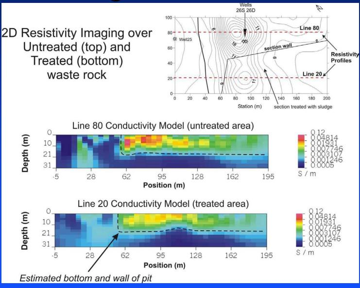
Challenges of Mapping Sludge Distribution Using Apparent Conductivity
