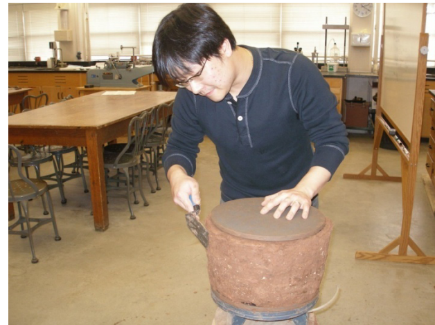
Trimming to the pedestal size
