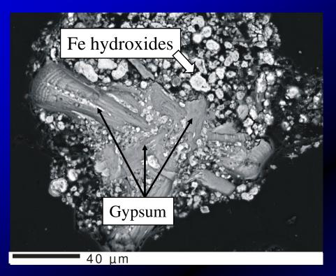
Fe hydroxide (<1 to 20 µm in size) is essentially pure with only minor amounts of other constituents (e.g. Mg, Al and S).
