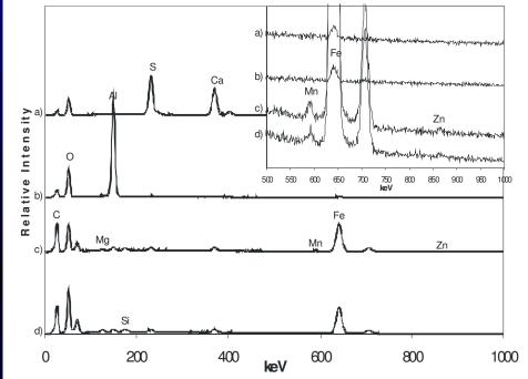
Fe hydroxides: (1-20 µm) well rounded grains that display compositional zoning Zn and Cu associated with Fe hydroxides (spectra c and d) and not gypsum (a) or Al hydroxide (b)
