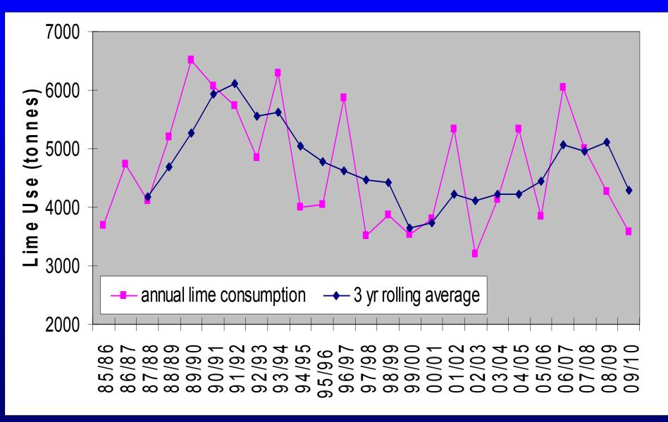
Annual lime use increased with waste rock production, decreased after soil cover construction and increased after the Main Zone pit lake reached its present height and the rebound in the water table.
