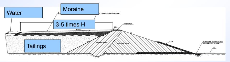
Construction of a beach upslope of the dam moves erosive wave action away from the dam and the hydraulic gradient is lowered – increasing the safety factor. Till was used as the beach material for this dam in Sweden (Lindahl 2008). At Huckleberry, the beach to prevent wave action against the dam is constructed from desulphurized tailings and use of a pit to expand the impoundment reduced the required dam height.
