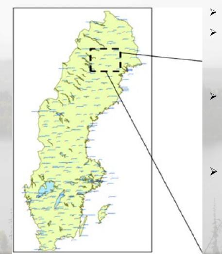
> 67° N (sub-arctic climate,  $T_{avg} = -1°C$ ) Pit lake: 279 ha 525 m deep 579 M m<sup>3</sup>  $Z_{r} = 28\%$ Main inputs: TSF runoff/seepage Waste rock runoff/seepage Natural runoff Pit wall runoff Direct precipitation to pit lake surface. Fill scenarios modelled: **Passive Fill** Slow fill - delayed pit lake overflow to realize water quality improvement of waste rock seepage
