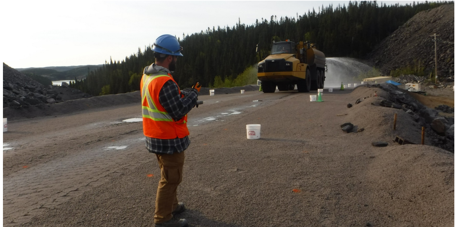
Large scale infiltration tests (J. Dubuc)
