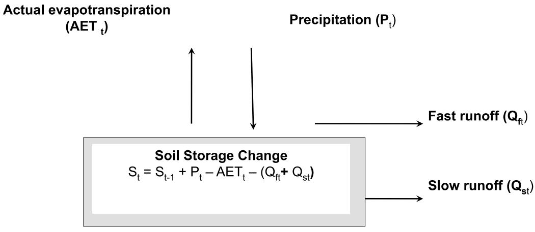
$S \downarrow t = S \downarrow t - 1 + P \downarrow t - AET \downarrow t - (Q \downarrow ft + Q \downarrow st)$
