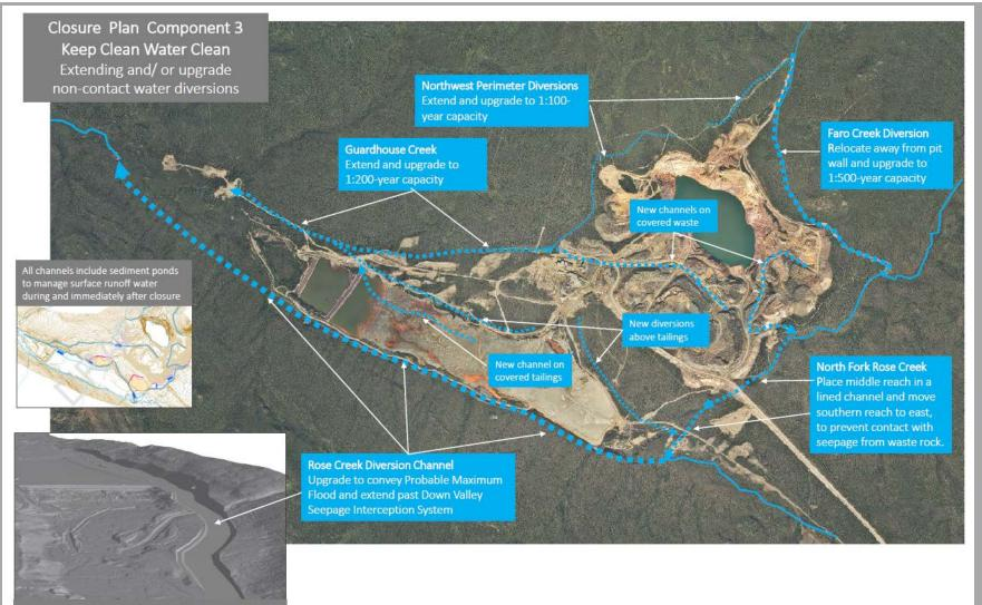
Schematic view of extended Rose Creek Diversion Channel
