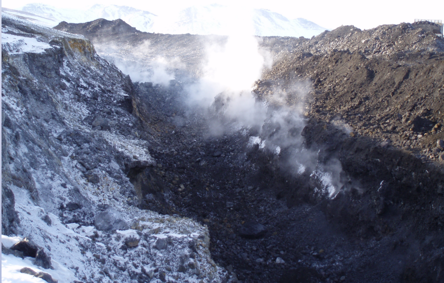
Trench dug to expose burning waste rock
