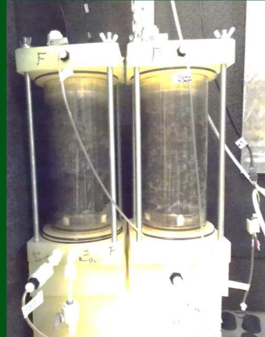
Customized test columns for waste rock developed in-house with  $O_2$ ,  $CO_2$ , RH & temperature sensors
