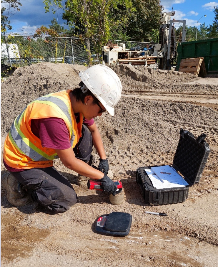
Magnetic Susceptibility Testing for ZVI content
