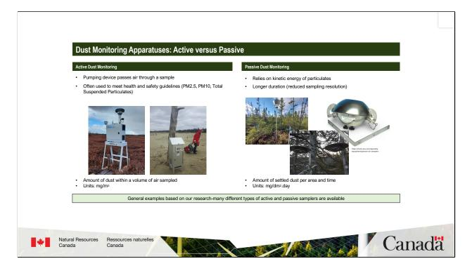
Notes: Before we dive into details and some case studies, I'll give an overview of the available dust monitoring devices. Dust monitoring can be grouped into 2 categories, one being active dust monitoring where a pumping device is used to pass air through a sample. These devices are often used to meet health and safety guidelines such as PM2.5, PM10 and total suspended particulates. Results are often presented as the amount of dust within a volume of air (m<sup>3</sup>).
