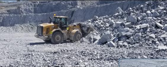
Identified freshly blasted mine blocks of the desired lithology and PAG/NAG classification
