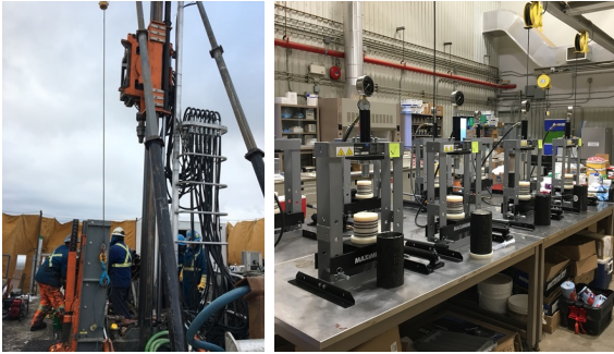
Amphibious sonic drill rig (left) and porewater squeezing setup (right).
