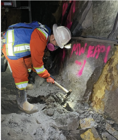
Muck sampling: assessment of material to be rinsed
