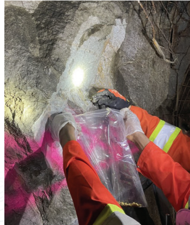
Precipitate sampling: assessment of solubility controls on metals/metalloids
