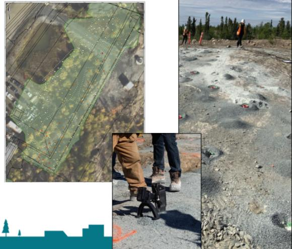
Part of the QA?QC system is the use of pXRF to measure tot S and As in drill cuttings on drilling grid.
