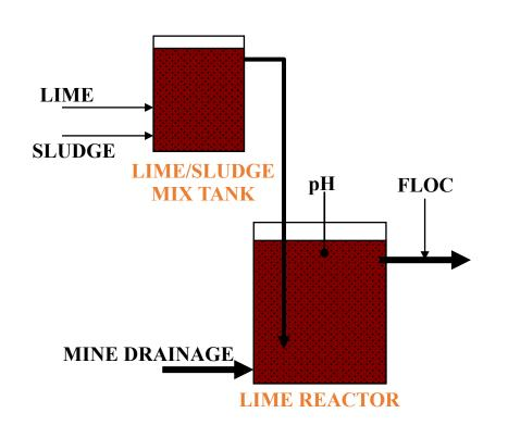
Injected Sludge, Lime, and Floc lines all risk plugging (worst is Lime/Sludge Mix)
