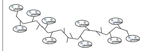
FLOCCULANTS ARE LONG POLYMER CHAINS WITH CHARGED "LIGANDS" THAT ATTRACT PARTICLES TO MAKE A HEAVY "FLOC" THAT SETTLES QUICKLY
