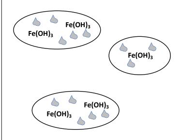
WITH A COAGULANT, THE PARTICLES MEET AND FORM LARGER PARTICLES
