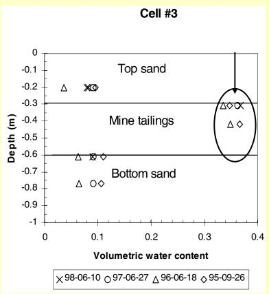
Well developed Capillary Barrier Effects
