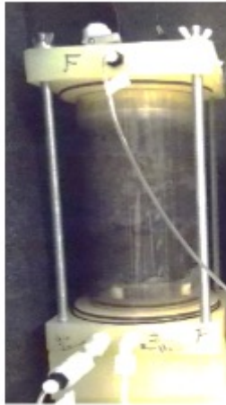
Figure 1 Photograph of the experimental setup, including custom-made columns with connections for water and gas flow.
