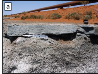
Magnesium carbonate hardpan formed at Mount Keith Nickel mine during carbonation experiments (Power et al., 2021).
