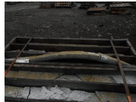
Expansion of drill core from conversion of anhydrite to gypsum (photo by Ed Saunders)
