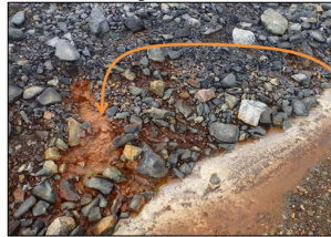
Image of pore clogging in low-flow seepage zone (Durocher & Robertson, 2019)
