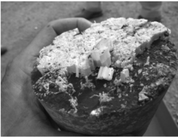
Observation of gypsum growth in bridge foundation (Alonso and Ramon, 2013)
